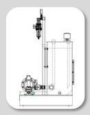
Dual pump pressure set point allows stall, single Coriolis feedback without heater or cooler
