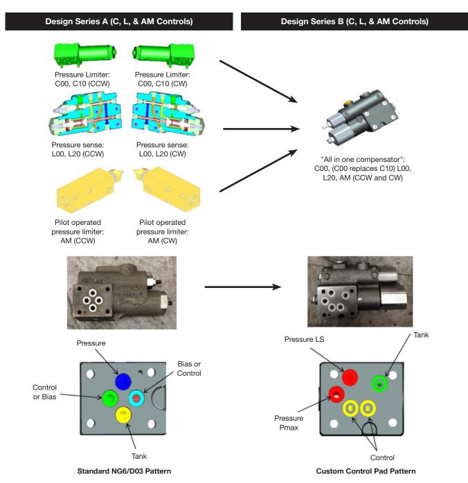
NOTE: Bolt pattern & size remains the same. No change to housing casting required.
