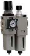
Filter/Regulator + Lubricator Combinations, poly bowl 5 micron element, 116 psig (8 bar) regulator + gauge and wall mounting brackets
