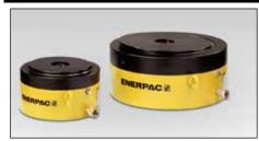
Model Cylinder Stroke Collapsed Height Number Class (tons) (in) (in) CLP-602 1.97 4.92 CLP-1002 100 1.97 5.39 CLP-1602 160 1.77 5.83 CLP-2002 200 1.77 6.10 CLP-2502 250 1.77 6.26 CLP-4002 400 7.01 CLP-5002 500 1.77 7.56
